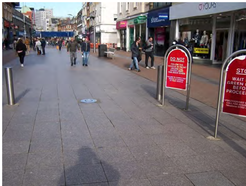
Figure 34: Route 19 impact point – rising bollards down allowing vehicle access
